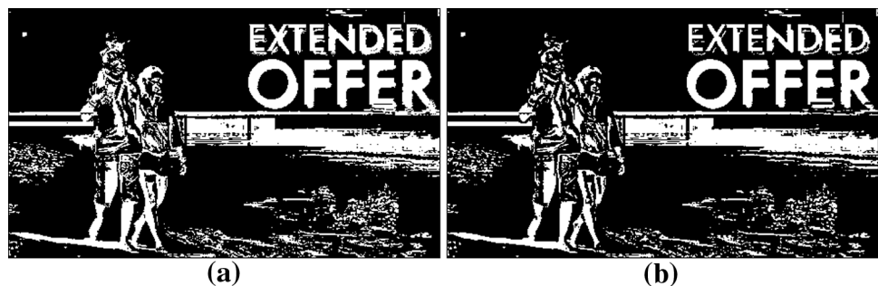
Fig. 5 a After binarization, text and non-text are connected, b text separated from non-text
