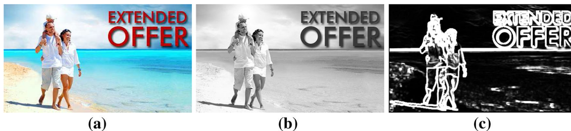
Fig. 3 a Input color image. b Gray image (Im), c variance map (VM) with n = 5
